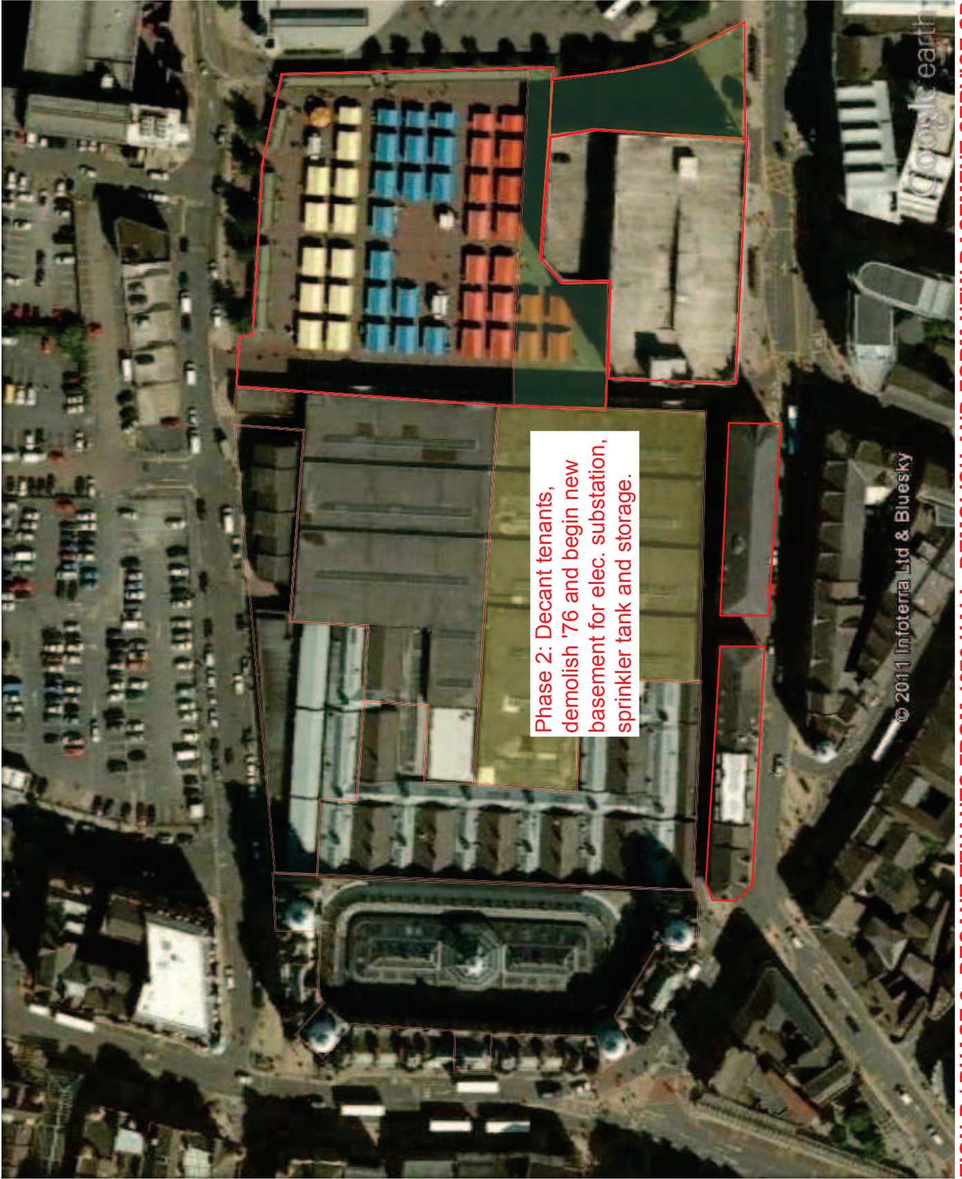
OPTION B / PHASE 2: DECANT TENANTS FROM 1976 HALL, DEMOLISH AND FORM NEW BASEMENT SERVICE SPACE
